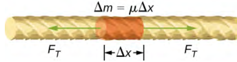
Figure 16.13 Mass element of a string kept taut with a tension F_T . The mass element is in static equilibrium, and the force of tension acting on either side of the mass element is equal in magnitude and opposite in direction.
