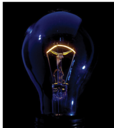
Figure 9.9 The incandescent lamp is a simple design. A tungsten filament is placed in a partially evacuated glass envelope. One end of the filament is attached to the screw base, which is made out of a conducting material. The second end of the filament is attached to a second contact in the base of the bulb. The two contacts are separated by an insulating material. Current flows through the filament, and the temperature of the filament becomes large enough to cause the filament to glow and produce light. However, these bulbs are not very energy efficient, as evident from the heat coming from the bulb. In the year 2012, the United States, along with many other countries, began to phase out incandescent lamps in favor of more energy-efficient lamps, such as light-emitting diode (LED) lamps and compact fluorescent lamps (CFL) (credit right: modification of work by Serge Saint).
